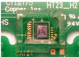
PR5201-CB are mounted on PCBs (standard/customized). A special assembly technique allows a quick assembly of the reticle.
